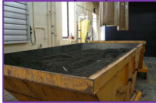
Washed Grit Ready for Disposal
